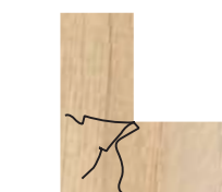
Cutting a laminate sheet at an angle of 90 degree leads to development of cracks. In corner after pasting. Therefore it is advisable to avoid cutting at an angle of 90 degrees.
